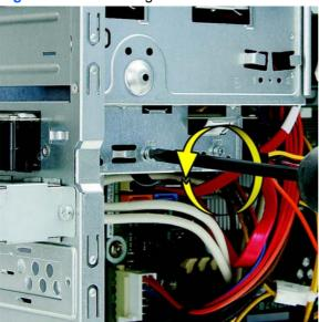
Figure 2-37 Removing the hard drive screws
